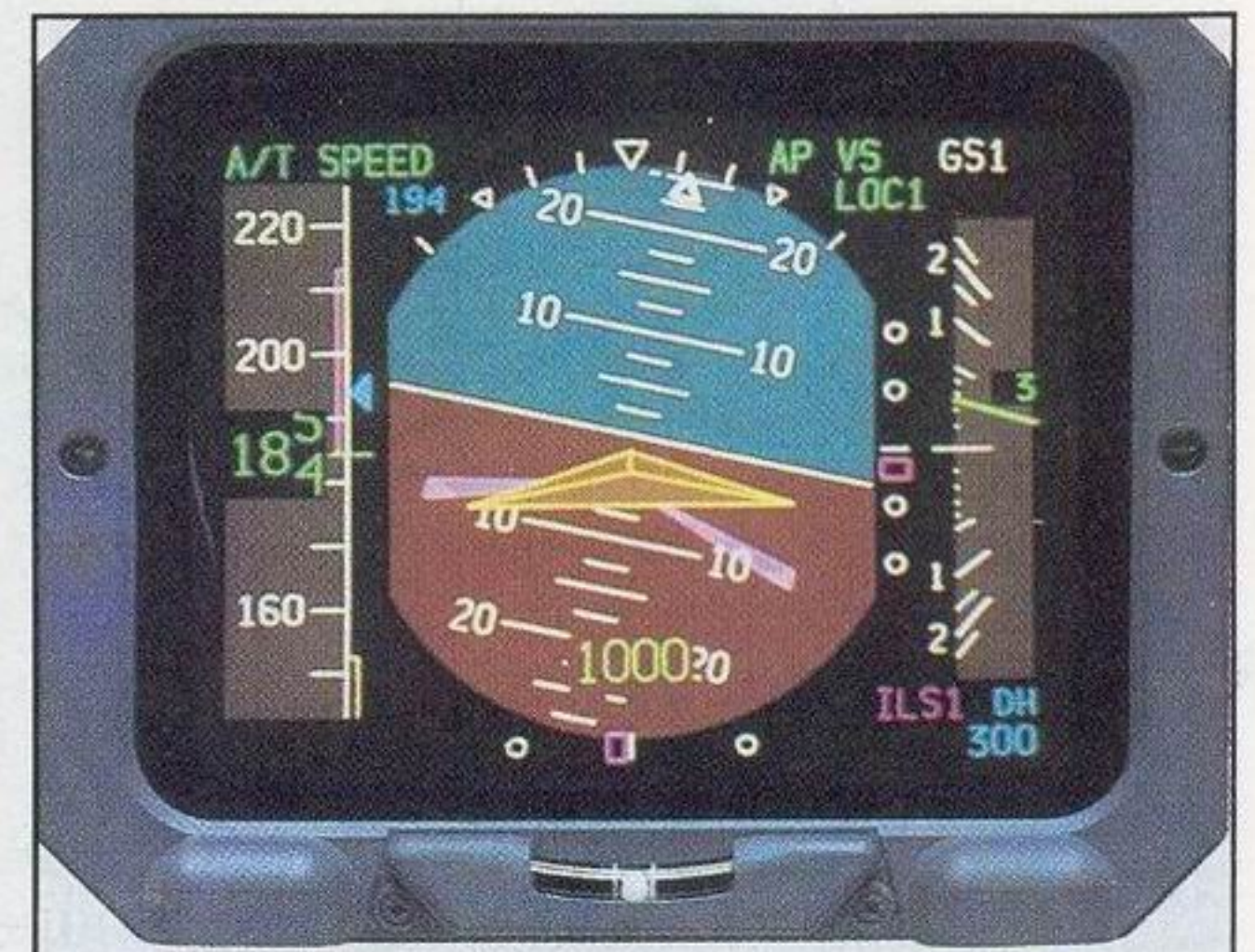
5" x 6" Primary Flight Display with airspeed and vertical speed side-scales.
