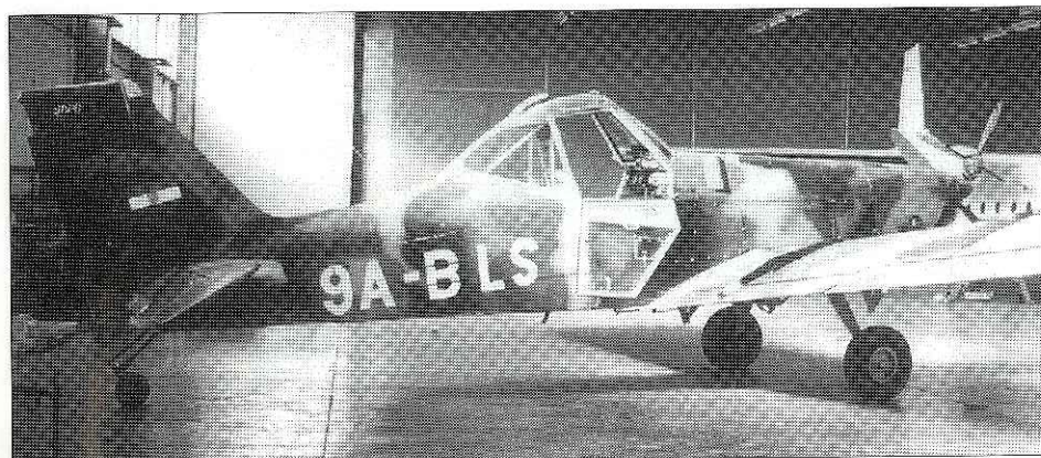
Wearing the newly applied civil registration of 9A-BLS is this Piper PA-36-300 Pawnee Brave. The aircraft wears a typical ZTC-applied camouflage scheme in Light Grey Green, Dark Green, Olive Drab and Chocolate Brown with Light Blue Grey undersurfaces. A Croatian flag sticker is worn on both sides of the fin, and a Piper logo remains visible on the top of the rudder. Formerly belonging to the civilian Privredna Avijacija Zagreb , this machine carried the former Yugoslav registration of YU-BLS, becoming RC-BLS in May 1992. The 9A- prefix was added two months later in July when the new registrations were introduced.
