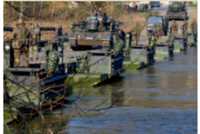
M3 Bridge Configuration
